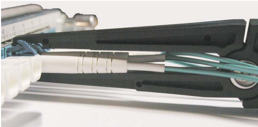
Figure 2: OPT SF-1 Gripping an LC Connector in a Dense Array (Note that the tips provide positive grip on the connector and release tab while not crimping fiber optic cables or connector boots.)
